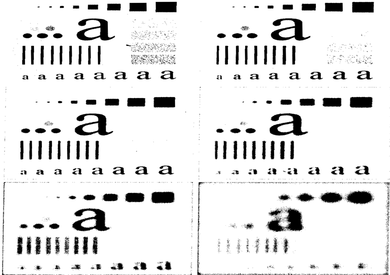
FIGURE 3.33 (a) Original image, of size 500 \times 500 pixels. (b)–(f) Results of smoothing with square averaging filter masks of sizes m = 3, 5, 9, 15, and 35 , respectively. The black squares at the top are of sizes 3, 5, 9, 15, 25, 35, 45, and 55 pixels, respectively; their borders are 25 pixels apart. The letters at the bottom range in size from 10 to 24 points, in increments of 2 points; the large letter at the top is 60 points. The vertical bars are 5 pixels wide and 100 pixels high; their separation is 20 pixels. The diameter of the circles is 25 pixels, and their borders are 15 pixels apart; their intensity levels range from 0% to 100% black in increments of 20%. The background of the image is 10% black. The noisy rectangles are of size 50 \times 120 pixels.
